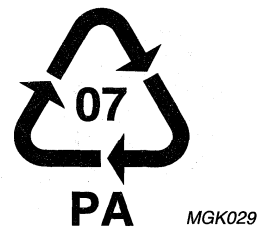
Fig.8 Other plastics. The acronym of the plastic is put under the recycling symbol. In this example: PA = polyamide.
